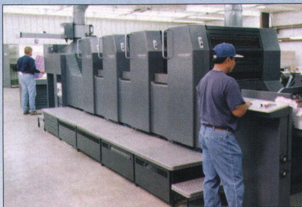
Newest (of 6 presses) Heidelberg Speedmaster 74, computer controlled with auto plate mounting & register
